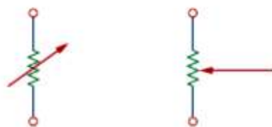
Figure 1.9 Circuit symbol for: (a) a variable resistor in general, (b) a potentiometer.
